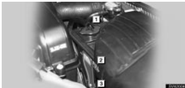
► 1 Reservoir cap 2 Upper line 3 Lower line
